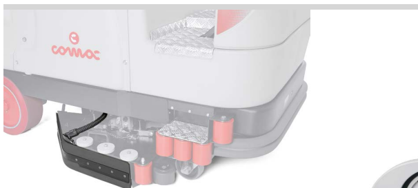
Suction system located on the brush head
