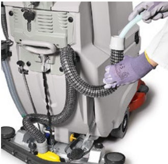
To ensure a perfect drying, the suction hose and the squeegee rubber blades must be cleaned at the end of any cleaning operation. The squeegee can be lifted to quickly clean the rubber blades
