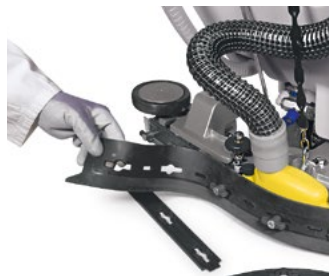
Rubber blades replacement or rotation are carried out in few seconds without any tools
