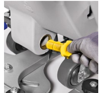
Solution filter cleaning
