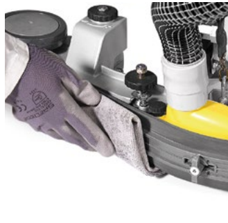
To ensure a perfect drying, the suction hose and the squeegee rubber blades must be cleaned at the end of any cleaning operation. The squeegee can be lifted to quickly clean the rubber blades
